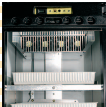
Fans provide 'Laminar Airflow'
