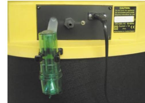
Fig. 5: Separate oxygen and nebuliser ports.
